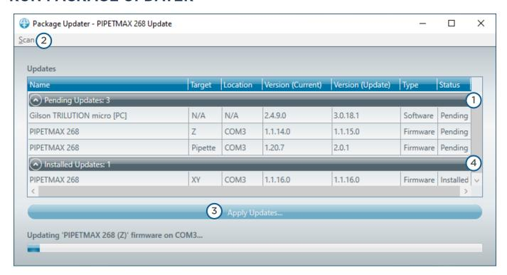
The Package Updater updates PIPETMAX software on the tablet or PC and firmware (if connected and necessary).
